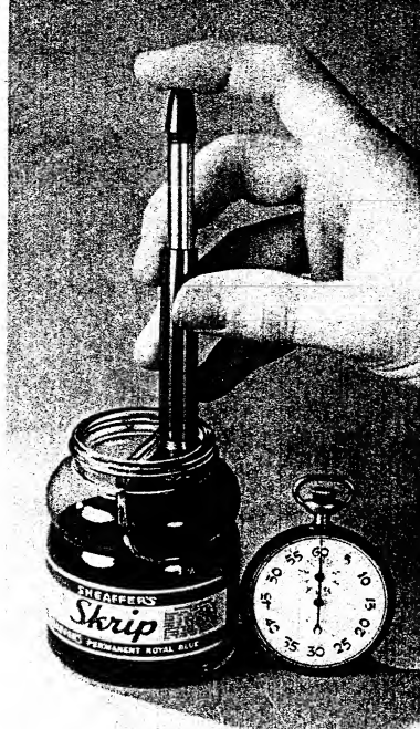
FINGER-TOUCH PLUNGER extended, pen is about to be touched into writing fluid. Stop-watch is poised, ready to record actual time consumed in operation.
